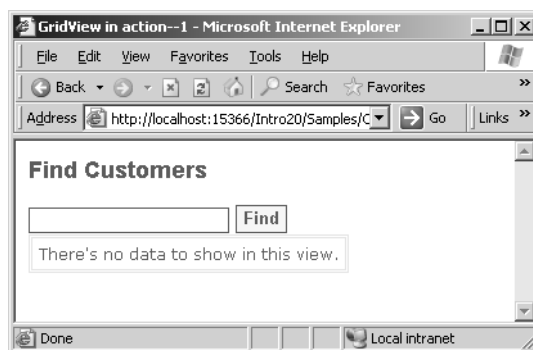
Figure 7-7 The GridView in action on an empty data source
