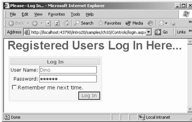
Figure 10-7 The Login control in action
