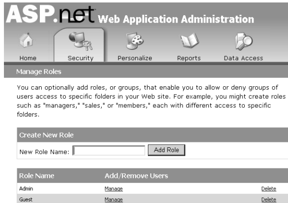
Figure 10-6 Using the Web Application Administration Tool to define the roles recognized by an application
