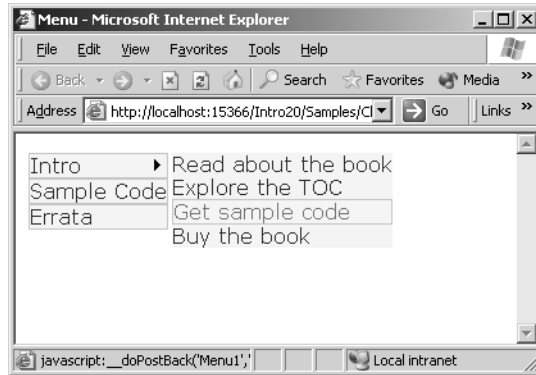
Figure 7-5 A simple Menu control in action
