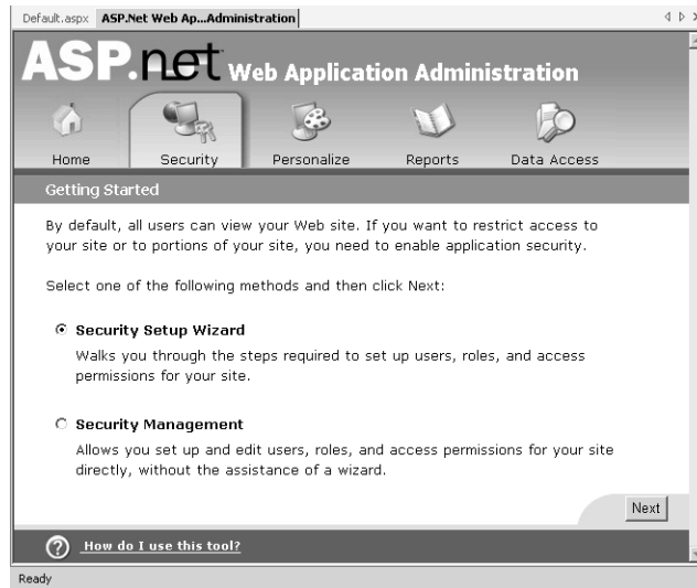
Figure 4-2 The ASP.NET Web Application Administration tool in action
