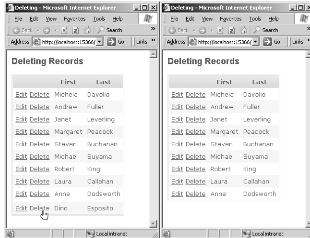
Figure 7-12 When the user clicks the Delete button, the underlying data source is invoked to physically delete the corresponding record.
