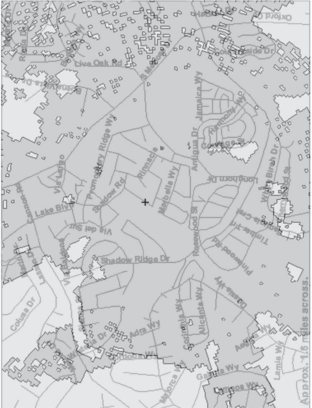
Figure 4-4a: Propagation model output plots terrain only
