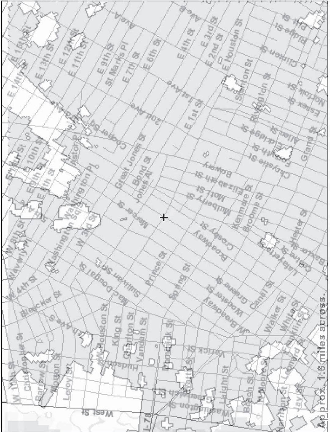
Figure 4-2a: Predicted Manhattan coverage based upon terrain only
