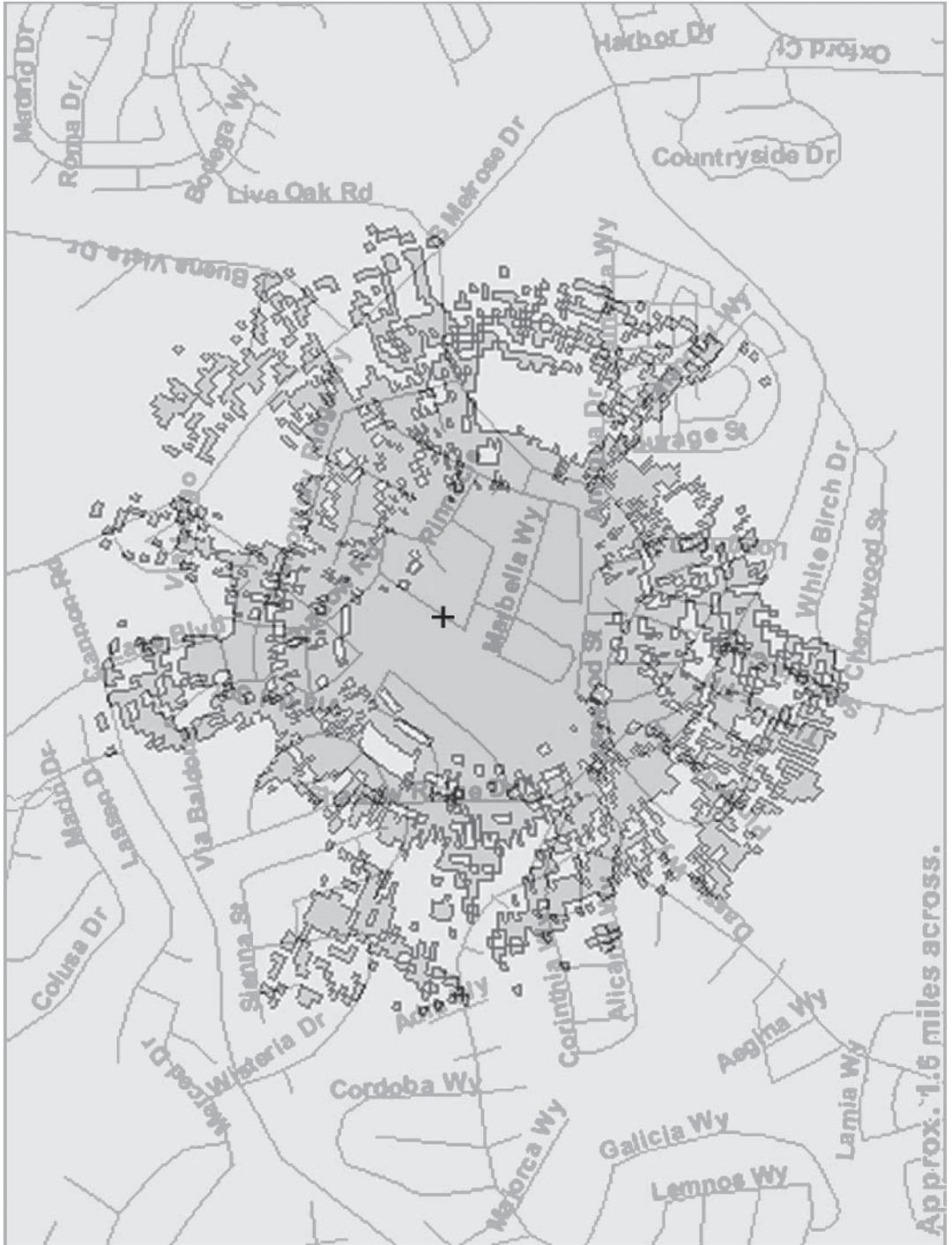
Figure 4-4c: Propagation model output plots terrain plus low density suburban morphology
