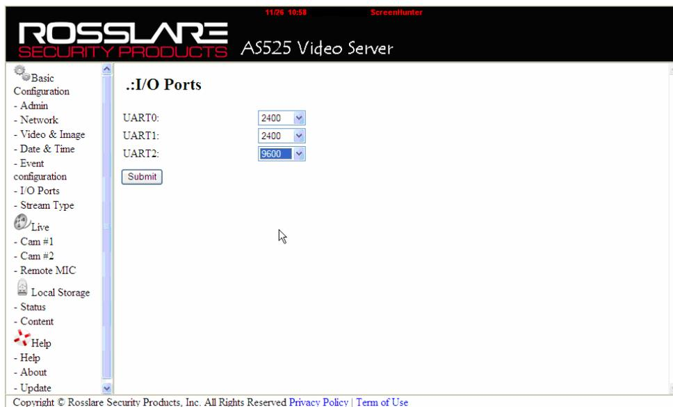
**Figure 28: I/O Ports Screen**
