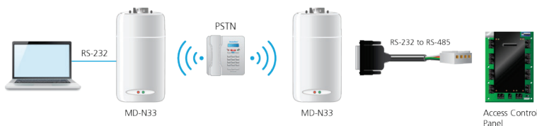
Figure 21: Remote Site Modem Configuration
